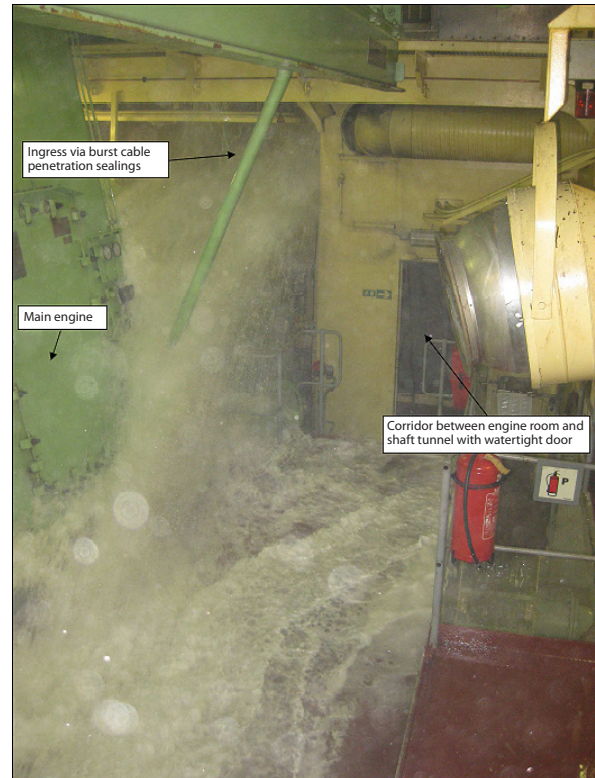
Figure 7: Ingress of Water into Engine Room. (Source: DMAIB, 2013)
