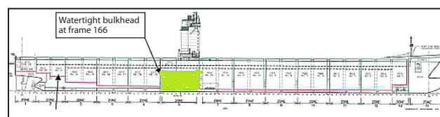
Figure 4: Longitudinal Section of Emma Maersk. (Source: DMAIB, 2013)
